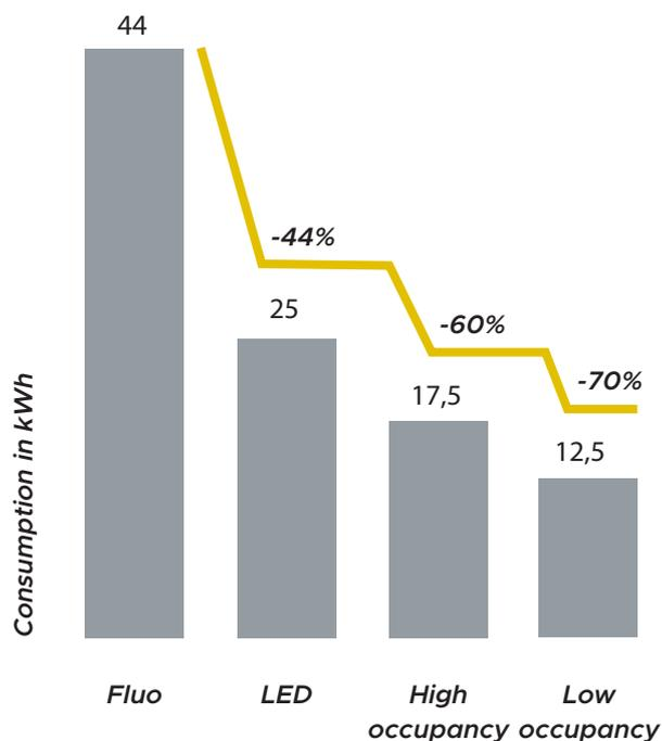
The installation of LED lighting allows installed power to be reduced by over 40% compared with the old 2x49W fluorescent solution.
