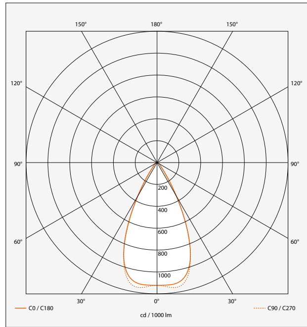
Semi-intensive light distribution LOR 96 %
